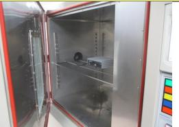
3. High Temperature/ Humidity Test Low Temperature Test
